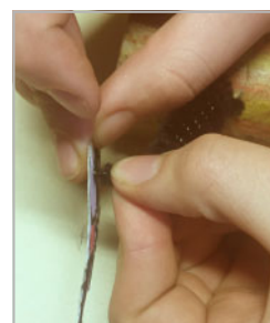
11. Thread spring through hole and twist to secure.
